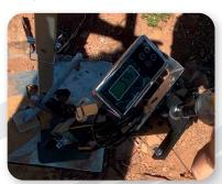
Step 8: Record uplift test on Load Test Document.
