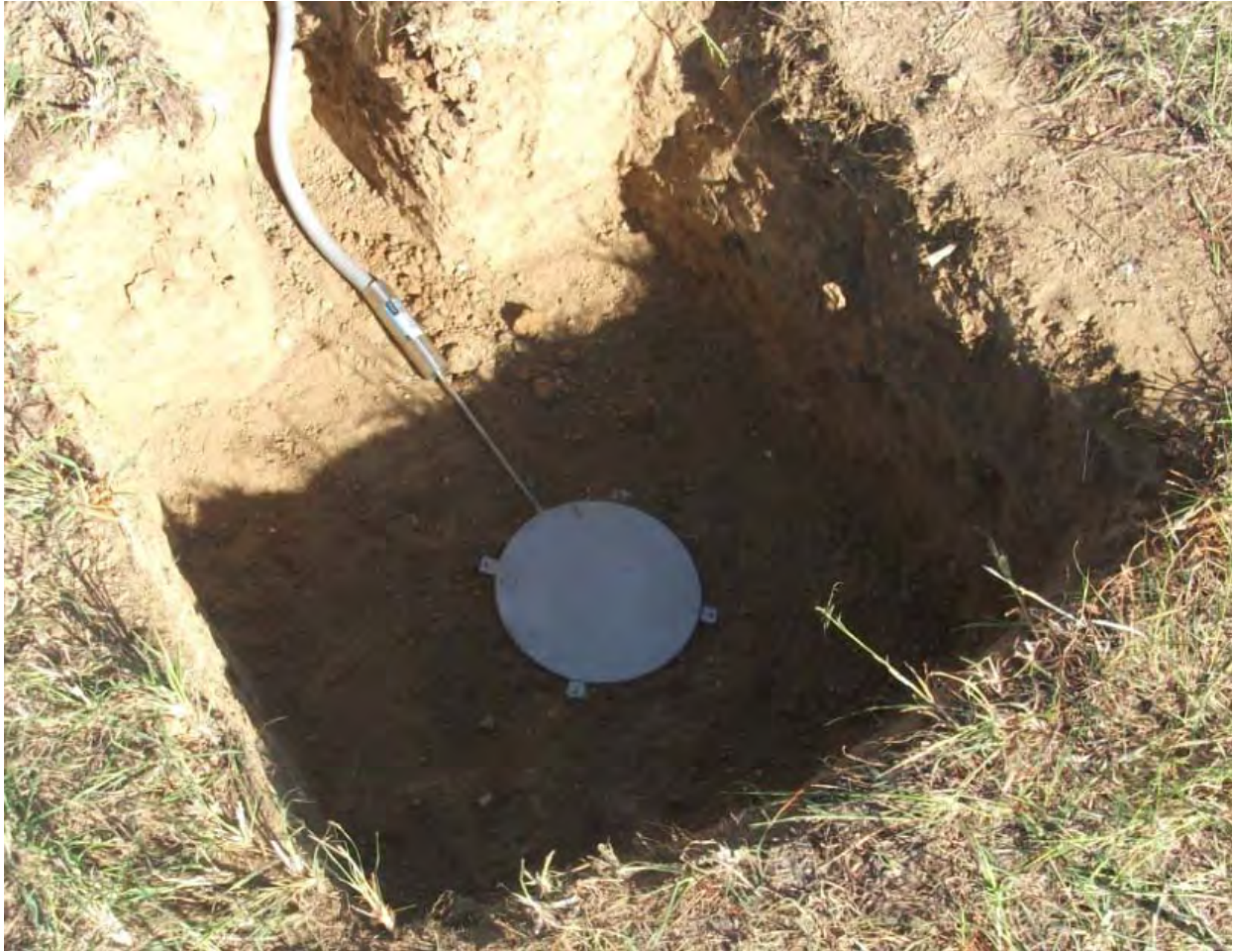
Photo 2: Geokon Earth Pressure / Load Cell Placed Inside a Trench
